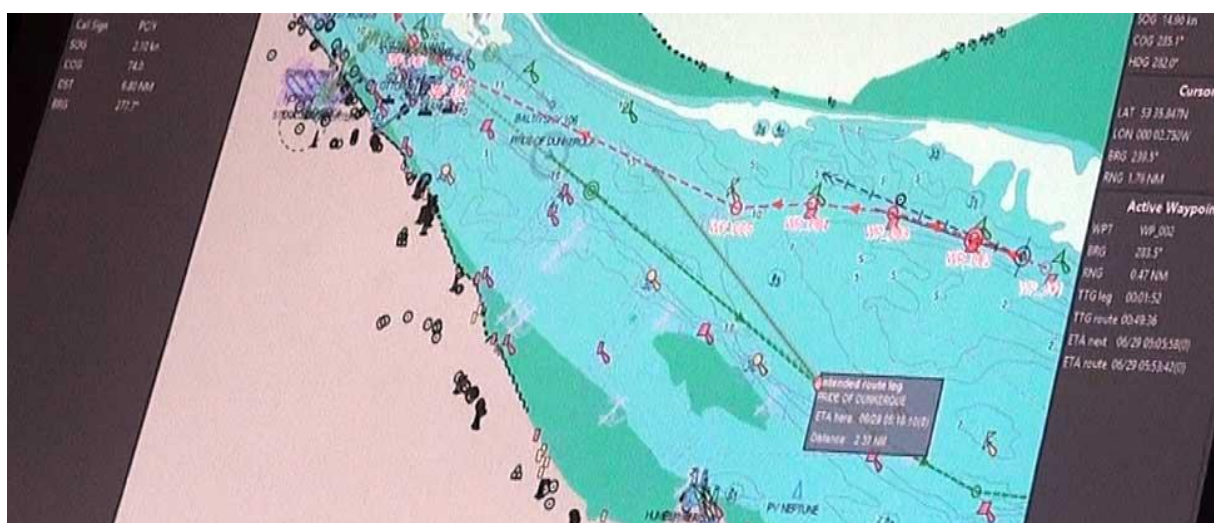
Figure 15: A screen shot from the updated HMI with the Intended route highlighted in darker green. The ship's present position is also highlighted with a circle and the bearing line connecting own ships position when the queried ship is at the position of the cursor.
