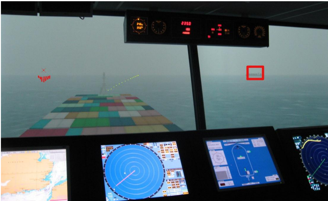
Figure 5: Sketch of augmented reality, showing dangerous target, area to be avoided and route suggestion
