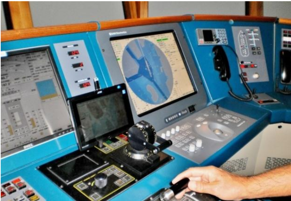
Figure 15: Portable Setup for Prediction Display on ECDIS in Monitoring Tool on Students Laptop on a Full-Mission Bridge of a Ship handling Simulator– the prediction is controlled by the Bridge Handle. The dynamic prediction shows the future manoeuvring track whereas on the Radar Screen the static path prediction shows still a straight line according to the initial conditions of the ship
