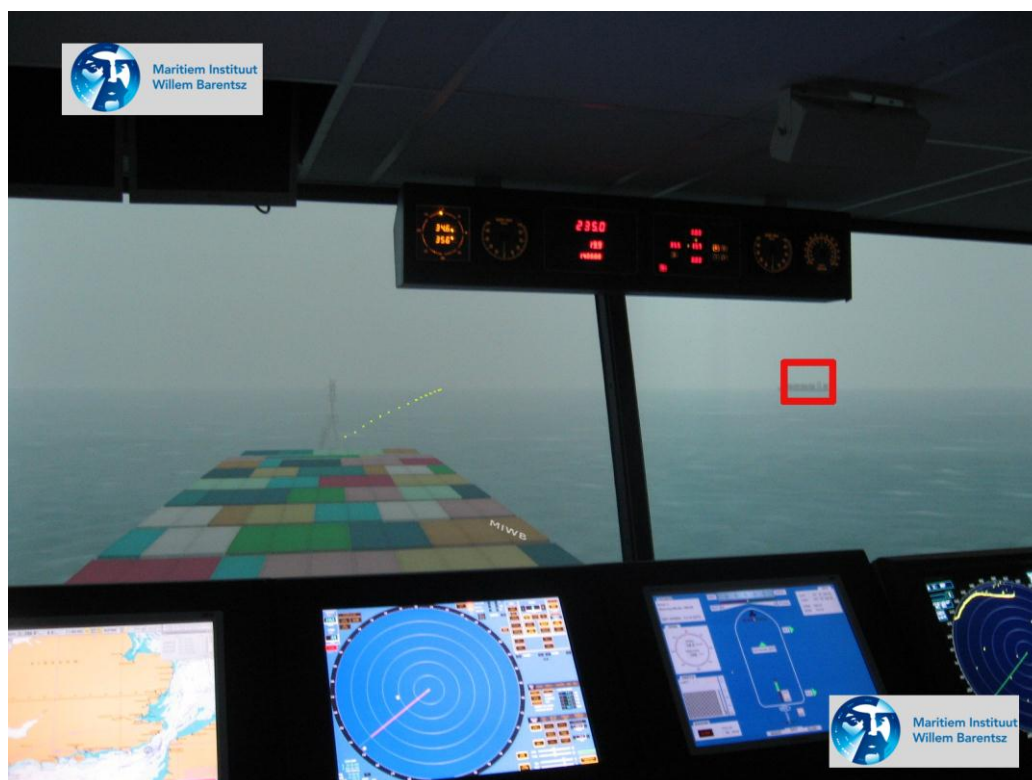
Figure 13: Conceptual Study for display of a vessel's route based on the RTM data to the bridge team using Head-Up-Display display mode (dotted line)
