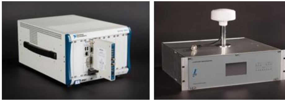
Figure 23 – R-Mode Modulator (left) and Rubidium clock (right) used in the test.
