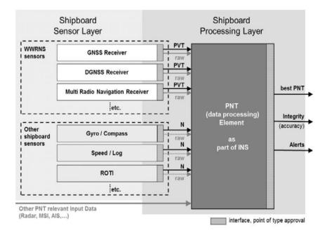
There are sensors for each data source which feeds the data it receives into the processor. The processor uses an algorithm to make a decision on what is the source of PNT with the most integrity; it then makes a decision of how to do to inform the mariner.
