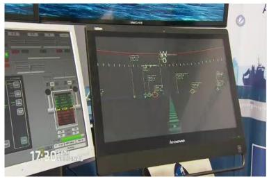
With the black background replaced for the view outside the goggles. This picture includes heading, AIS information and other symbols with colours based on urgency.
