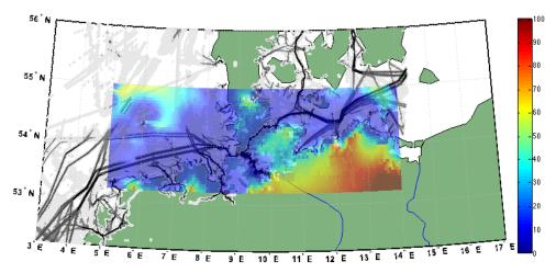
The next step was to build a transmitting site in Ijmuiden and Noordwijk to provide a transmission system testbed on MF. The first measurements were on the 27<sup>th</sup> of January. The results are very encouraging and validate the feasibility study that we could receive better than 5m accuracy.
