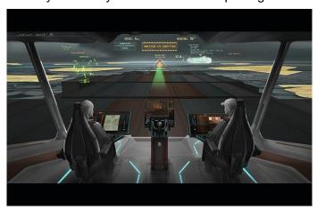
In this image you can see a version of augmented reality on the screen – displaying the ship's route, speed and other characteristics as well as the characteristics and routes of other ships.
