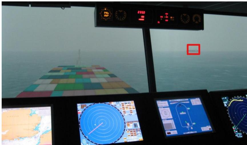
Figure 4-8. Indication of dangerous target projected as a red box on the bridge window.
