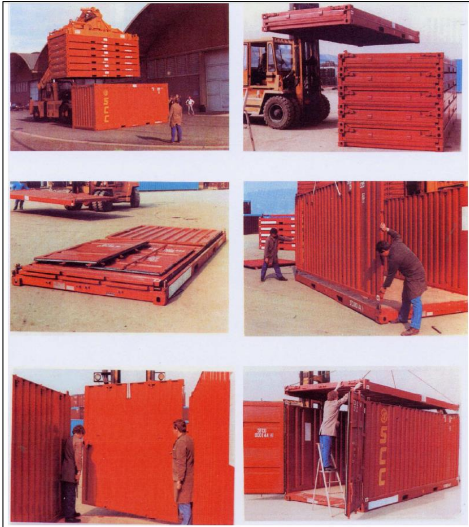
Figure 2. Stacking, transporting and opening foldable containers Source: Konings (2005)
