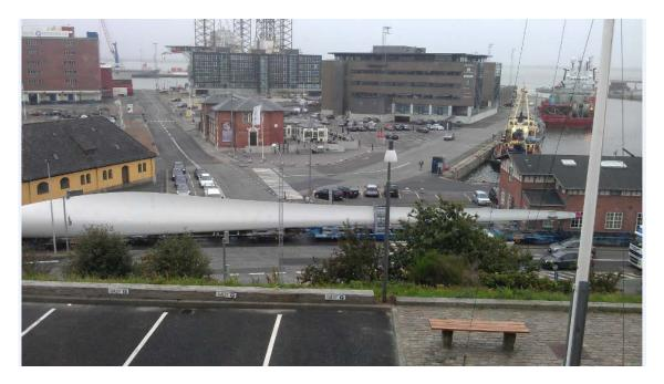
Above photo shows the transportation of a 55 m wind turbine wing on the existing track in the Port of Esbjerg. The photo demonstrates the possibility of using the current track for the transportation of large objects. By erecting a terminal in the new port area, we expect the number of such transports to grow significantly.
