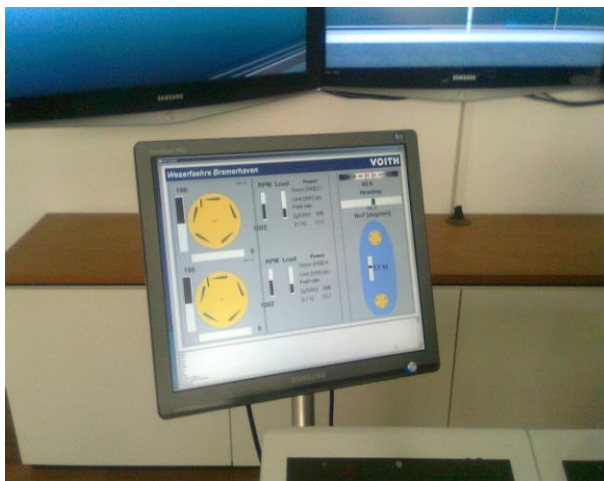
Fig.8: control display picturing fuel cons, pitch, speed etc.
