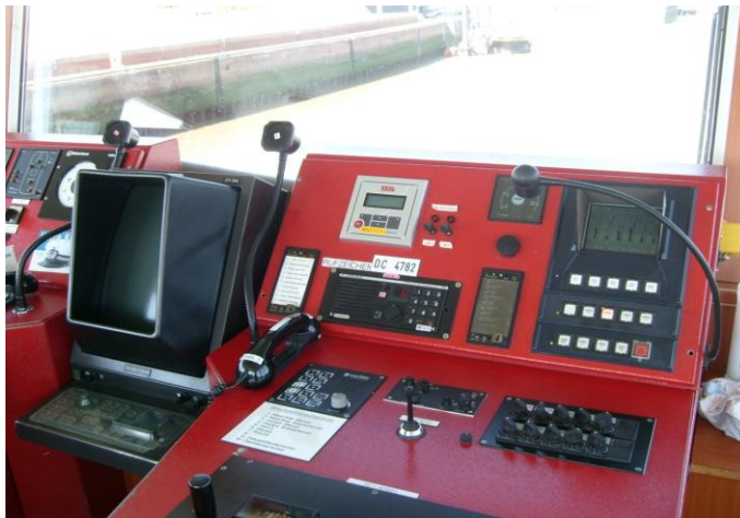
Fig.5: Digital gauge at the bridge (light grey box)
