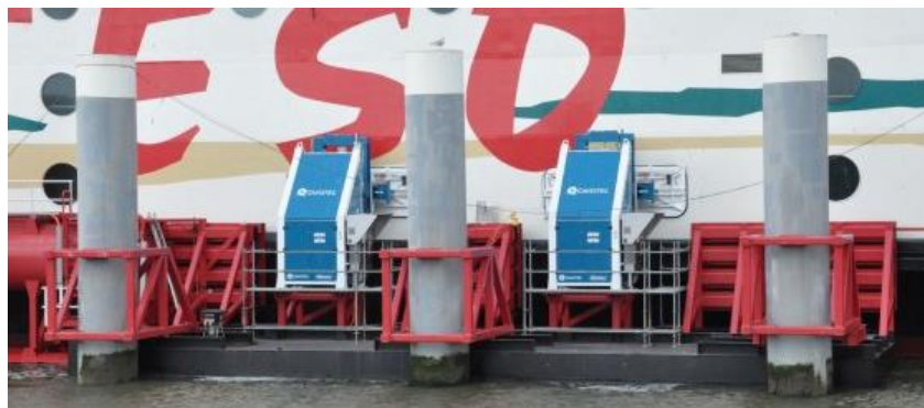
The new Cavotec auto-mooring system
