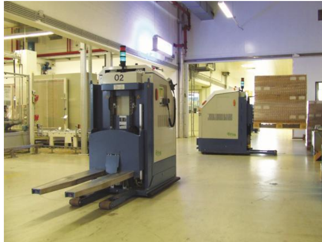
Figure 2.3: FROG AGV Industrial application
