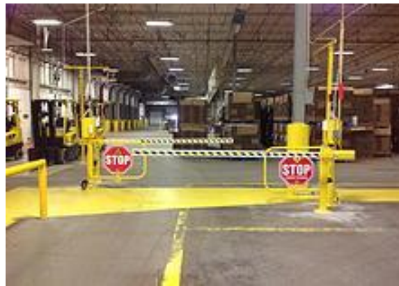
Figure 3.21: Marking to separate manned and unmanned vehicle areas
