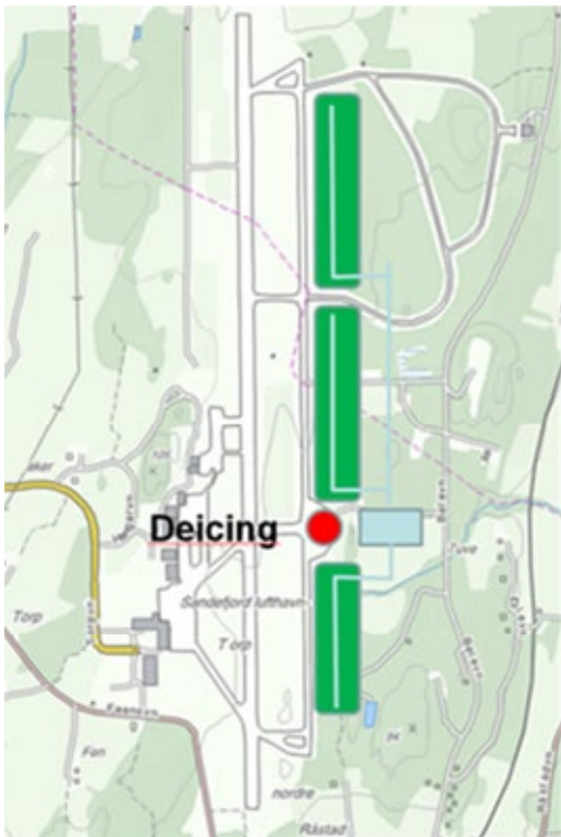
Figure 3: Balancing pond winter collection and green irrigation along taxiway
