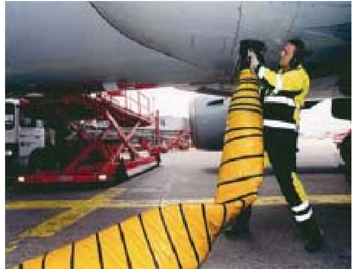
Figure 4, Connection Point for preconditioned air at the lower fuselage
