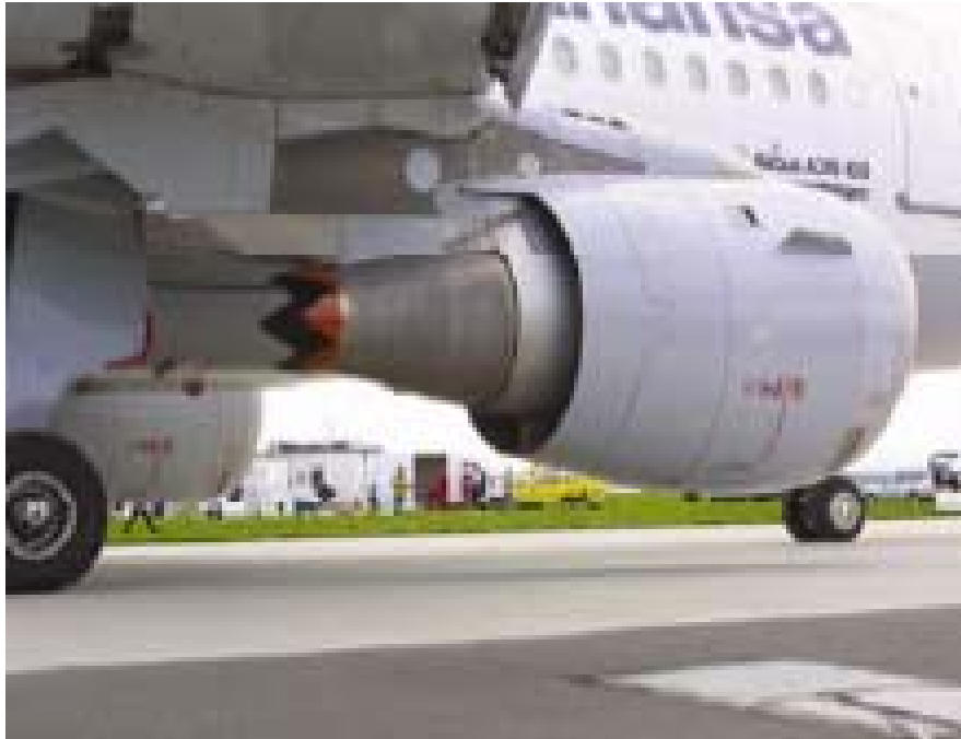
Figure 17, Serrated Nozzle Application on a CFM 56 Engine
