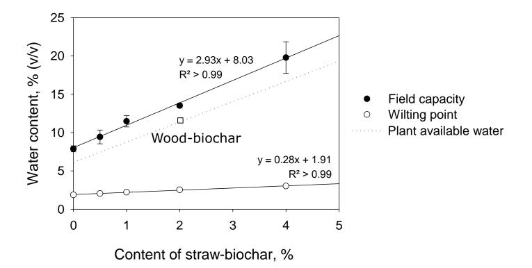
Volumetric water contents at 30-80 cm depth: in-situ values after drainage, values at the wilting point, and difference between the two. Average values and standard errors (n=3).
