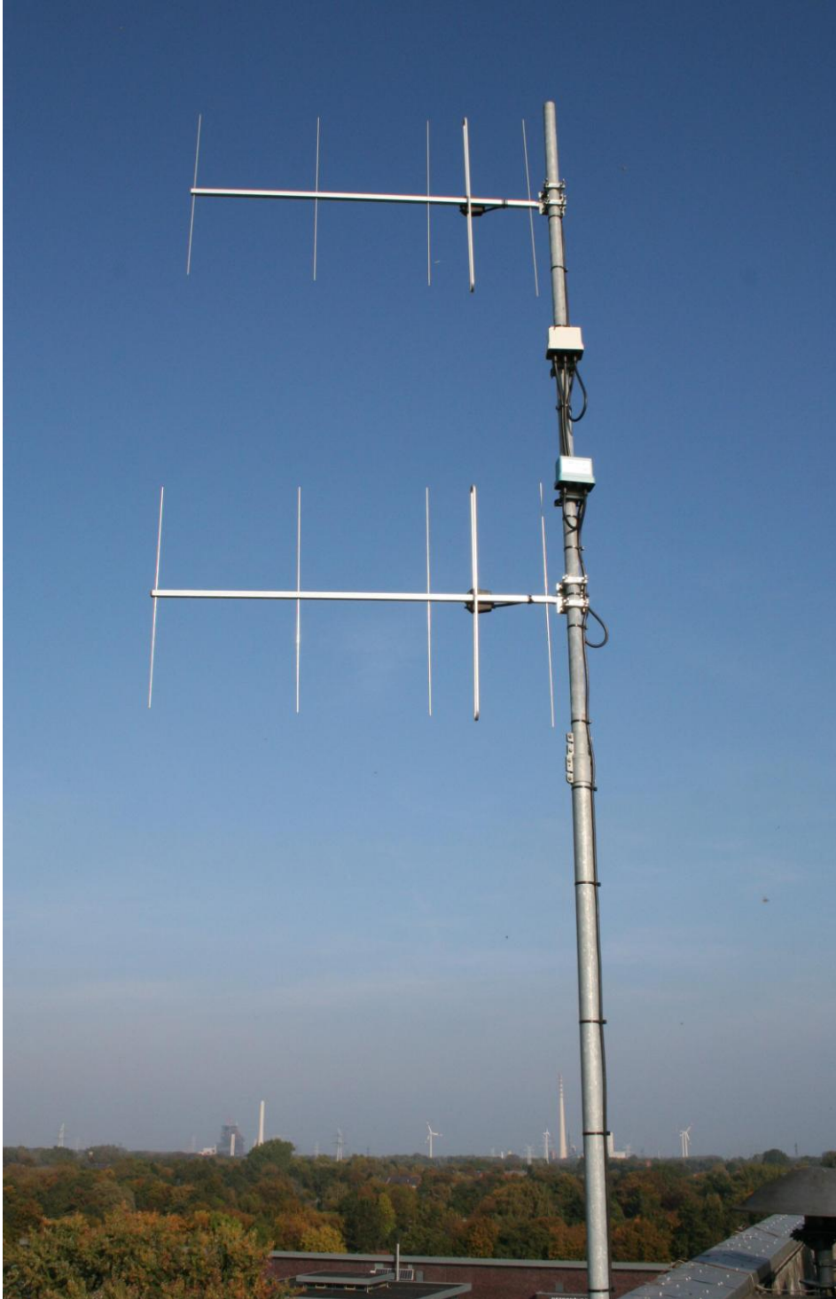
Picture 11 - Test Set-up of the Yagi Group Prototype
