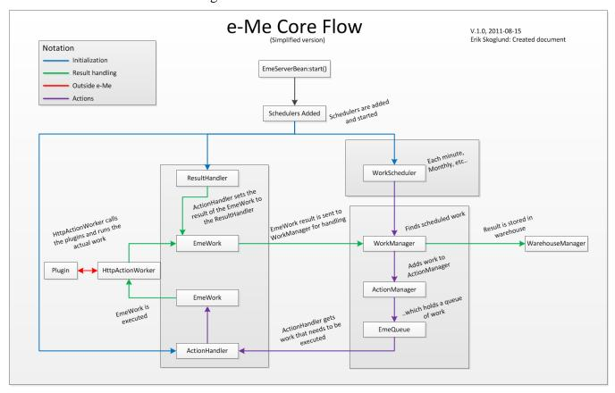
This image shows the flow of Core. Core is basically a machine running scheduled tasks, but it also relies on many plugins. These plugins are completely separate from Core itself and are deployed freely on the same server running Core.
