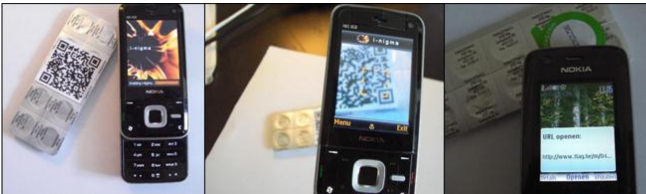
Figure 11. (a) QR code and Nokia N81 8GB, (b) Scanning the QR code, (c) Scanning the RFID tag.
