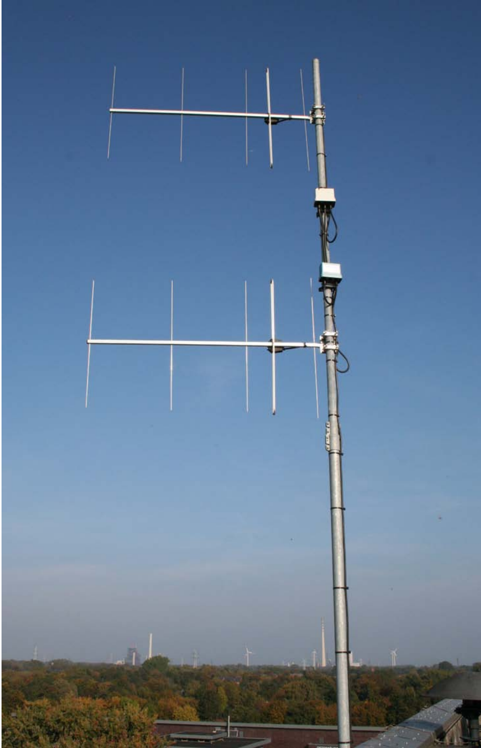
Picture 12 - Test Set-up of the Yagi Group Prototype
