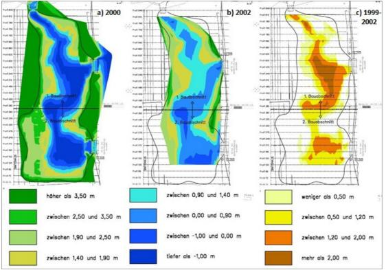
Figure 16: Topography and bathymetry (elevation in m NN) at Kleinensieler Plate: (a) in 2000; (b) in 2002; (c) difference between 1999 and 2002: largest difference in the deepest zones
