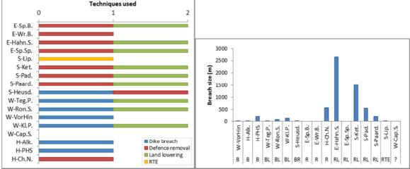
Figure 10: Overview implementation techniques used for the different TIDE examples (LEFT) and link between implementation technique and breach size (m) (RIGHT). Implementation techniques: dike breach (B), dike breach + land lowering (BL), dike breach + defence removal (BR), defence removal (R), defence removal + land lowering (RL), RTE.
