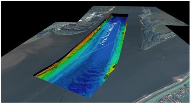
Figure 19: Position of the sediment trap at the river Elbe (source: HPA)
