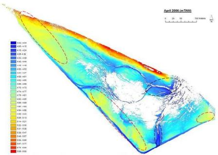
Figure 14: 3D-picture of the Paardenschor in April 2006 (m TAW). The red circled zones are low hydrodynamic zones, the black circled zones high hydrodynamic zones. (BRYS et al. 2005)
