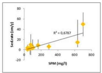
Figure 13: Correlation between SPM and the average sedimentation rate on the site ( $R^2=0,6787$ ; T=4,6; p<0,001).
