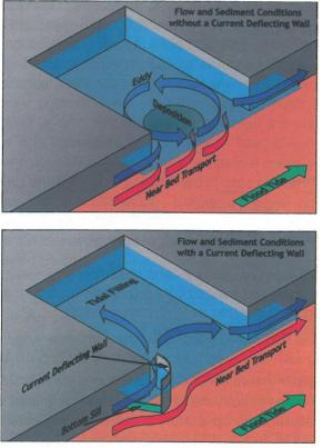
Figure 17: Scheme of current deflecting wall (PIANC, 2008)
