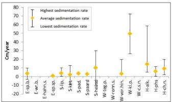
Figure 12: Average sedimentation rate per TIDE MRM with indication of the highest and lowest measured (or monitored) sedimentation rate as error bars
