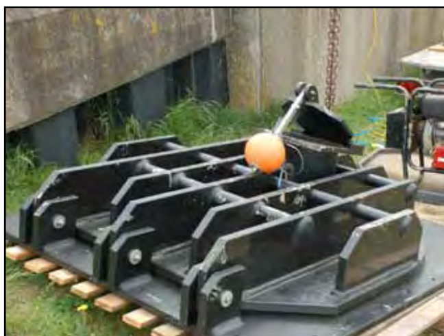
New HDPE tidal flap incorporating a "pet door" device awaiting installation on the Adlingfleet Drain, Tidal Trent, UK
