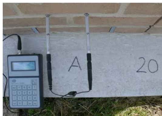
Measuring moisture on a test piece (GANN-DEVICE)
