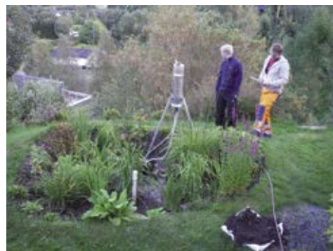
Testing infiltration intensity in rain garden in Melhus
