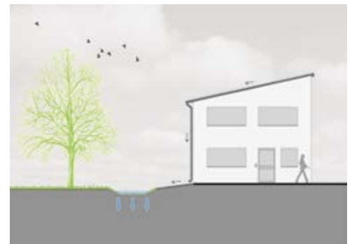
Stormwater run-off from a roof managed on plot using a swale for infiltration.
