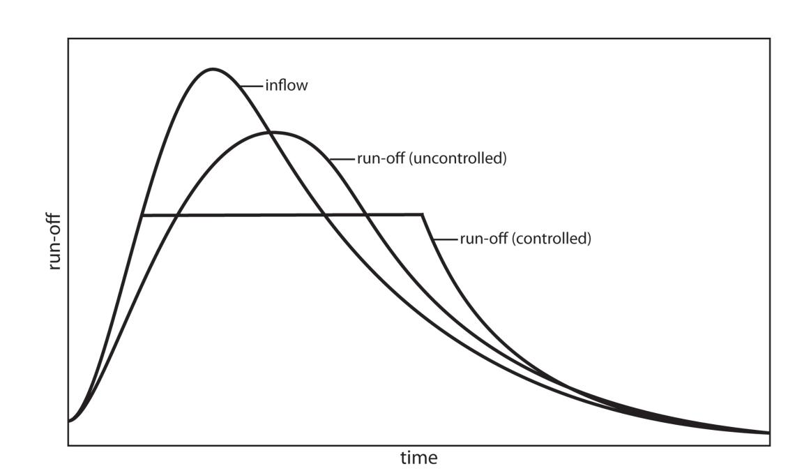
The retention capacity of the basins can be used best, if run-off-peaks of extreme flood events are cut precisely at the amount of discharge that can be managed safely.
