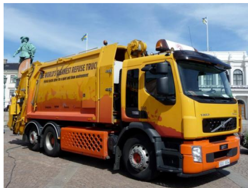
Hybrid refuse truck in Gothenburg. Heavy duty vehicles are the worst polluters, and hybrid solutions offer a possibility to drive silently and emission free in sensitive areas. Photo: Renova
