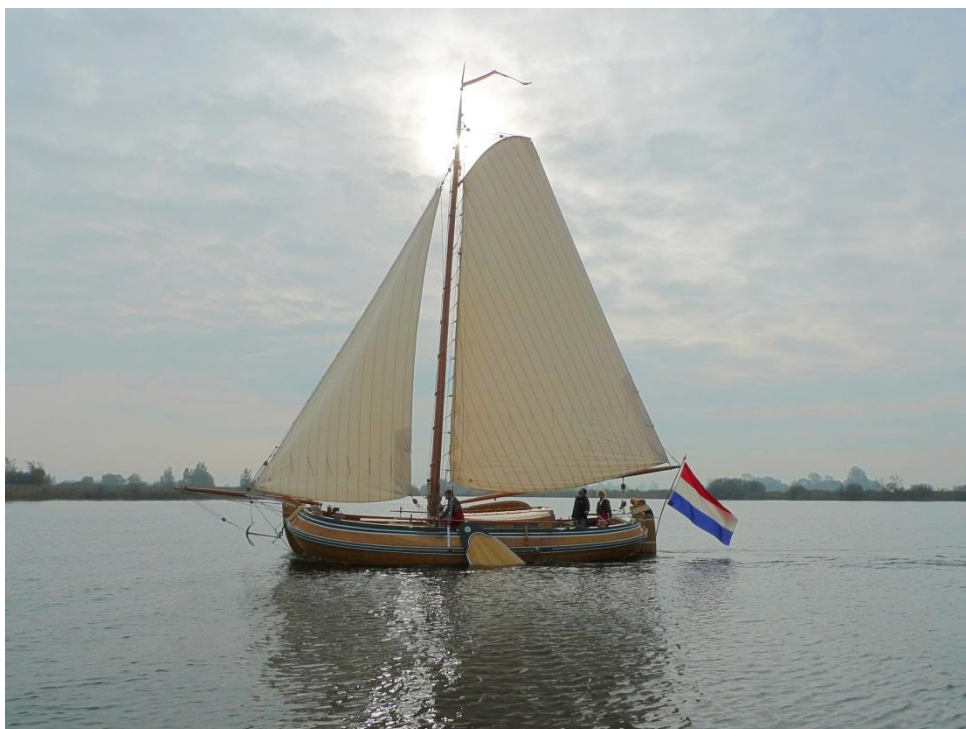
Traditional Dutch sailing yacht equipped with electric drive, ideal for inland waterways with slow speeds. Boats can more easily carry the heavy batteries thereby making the range between recharging a less critical issue. Photo: www.SEFF.nu
