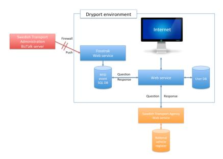
An open source RFID service platform, Fosstrak (<a href="http://www.fosstrak.org/">http://www.fosstrak.org/</a>), internally used by STA was implemented to handle the connectivity between the STA BizTalk server and the internal Dryport RFID event database. Fosstrak is entirely based on EPCIS standards (<a href="http://www.gs1.org/gsmp/kc/epcglobal/epcis">http://www.gs1.org/gsmp/kc/epcglobal/epcis</a>) developed by EPC Global.
