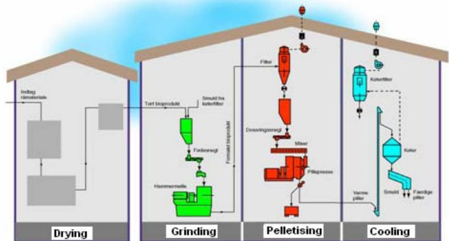
Figure 31: The pelletising process (Pellets@tlas, 2009)
