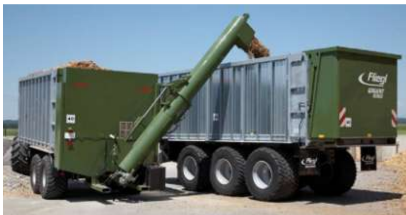
Photo 12: Auger discharge trailer (courtesy of Fliegl)
