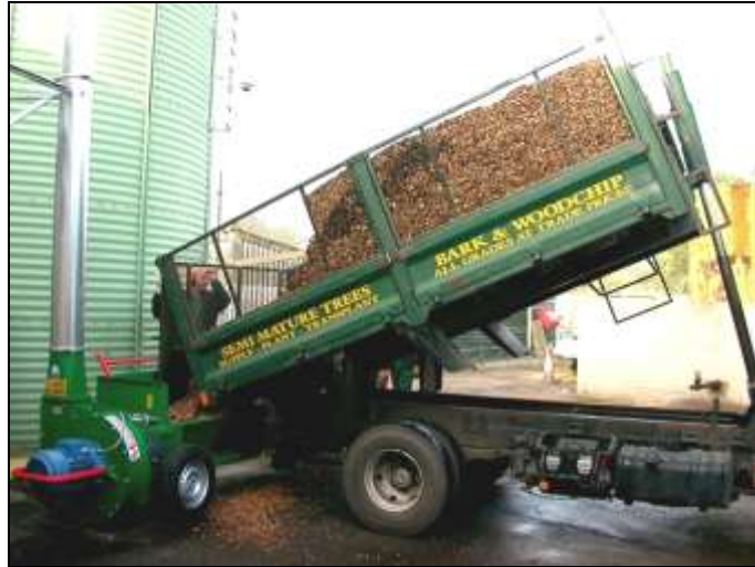
Photo 10: Customer based chip blower (courtesy of Practicality Brown)
