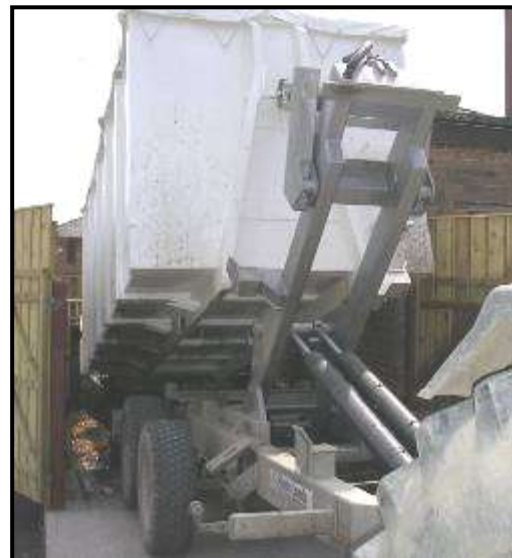
Photo 13: Hook-bin delivery system
