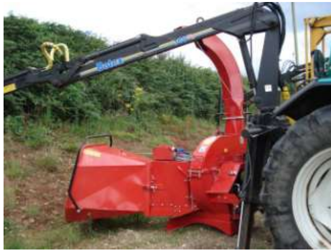
Photo 7: Disc chipper suitable for woodfuel production
