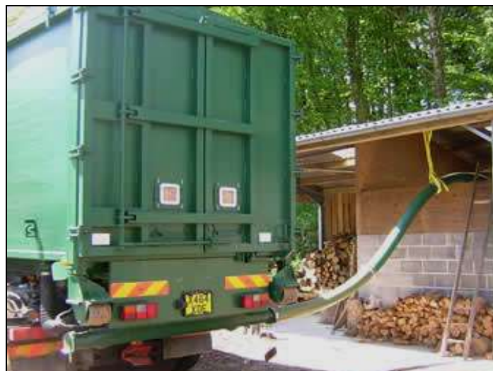
Photo 9: Specialist chip blowing lorry (courtesy of Forest Fuels Ltd)
