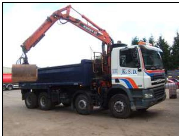
Photo 11: Clamshell grab lorry (courtesy of KSD)
