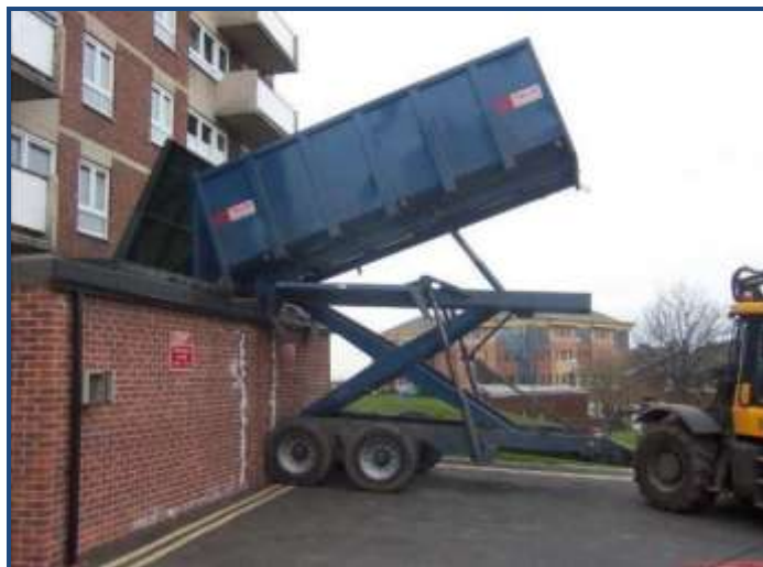
Photo 8: Example of a high-lift trailer loading into an above-ground store
