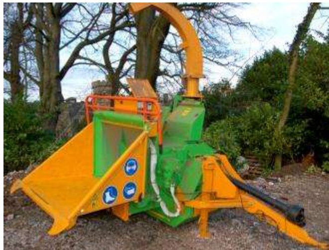
Photo 6: Drum chipper suitable for woodfuel.
