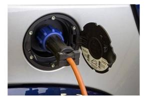
Figure 5 – Common plug used for charging an electric vehicle<sup>4</sup>
