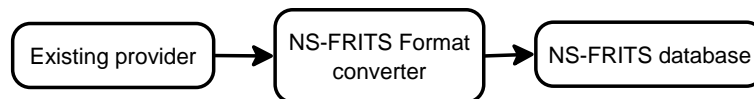
Figure 3.1 Illustrates how data from existing(independent) providers are inserted into the NS FRITS database
