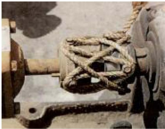
Figure 2.4: Temporary repair of coupling. How long will it work? (Source: SPM)
