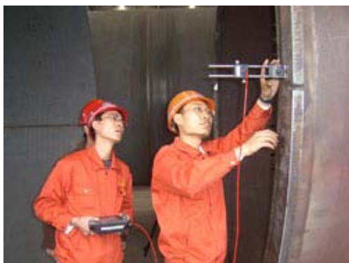
Figure 3:29 Flatness measurement of towers in a wind turbine and alignment of generator/gearbox (Source Damalini)
