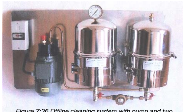
Figure 7:36 Offline cleaning system with pump and two filters
