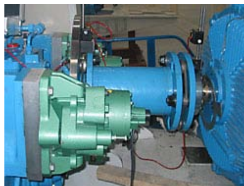
Figure 3:29 Flatness measurement of towers in a wind turbine and alignment of generator/gearbox (Source Damalini)
