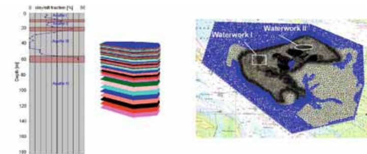
Fig.2. Hydrogeological model (Fig. left). Numerical model, setup with 39 vertical layers (centre of the figure), discretization of the model in 1 m depth (const. mass boundary conditions for sea water are marked blue) (Fig. right).
