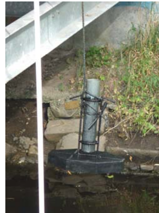
Sediment sampler at the Danish case study Harrestrup stream
