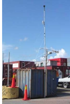
Sampling station for atmospheric pollutants
